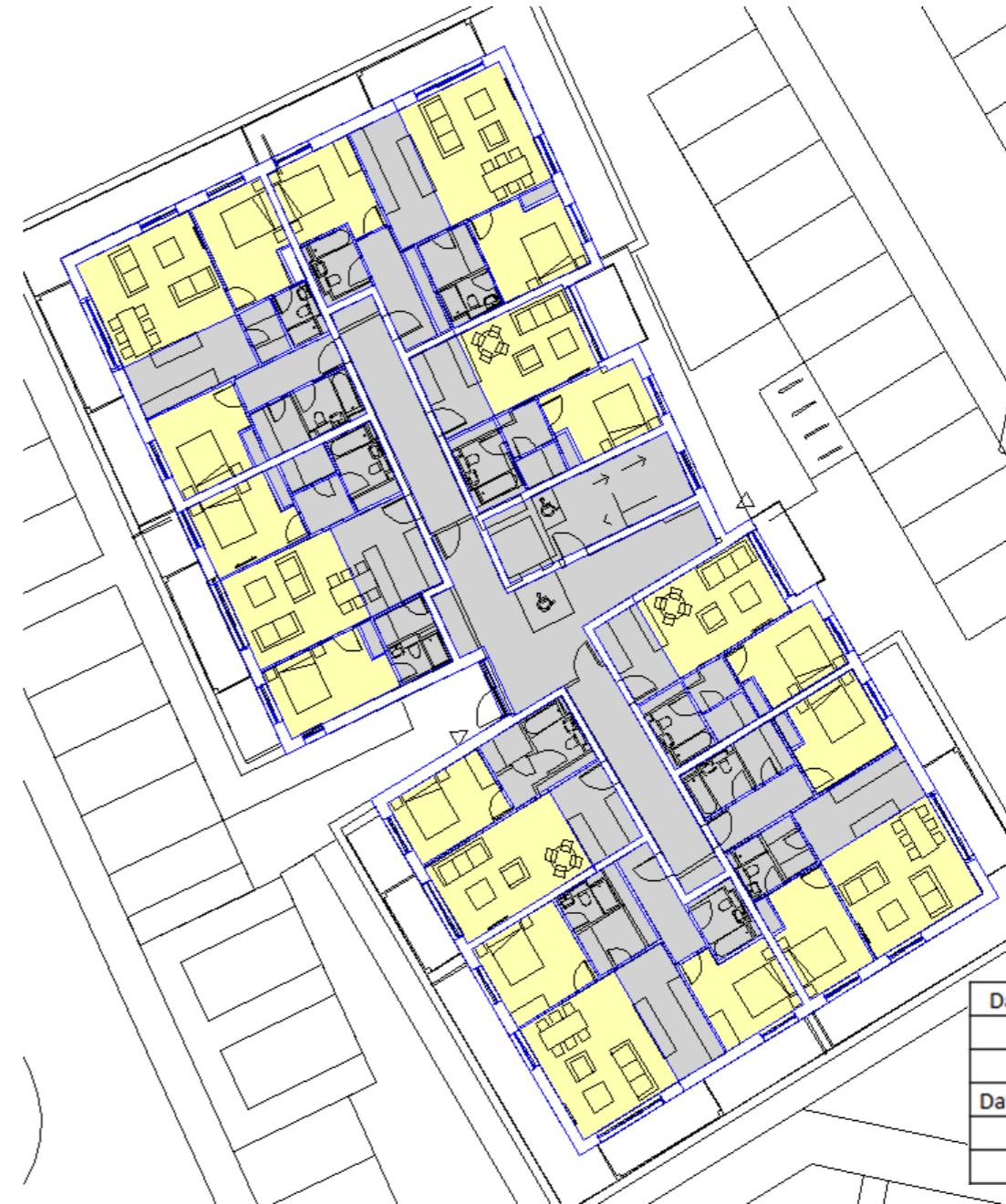
Fig 2.1.2.2 - Level 01 - Daylight Results - Pass/Fail
